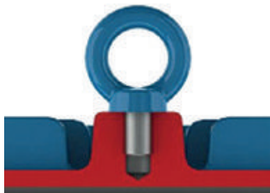
Figure 4.1 - Correct tightening of the eyebolt
