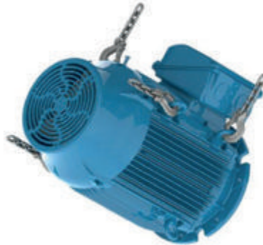
Figure 4.18 - Motor is being rotated to horizontal position
