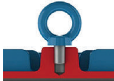
Figure 4.2 - Incorrect tightening of the eyebolt
