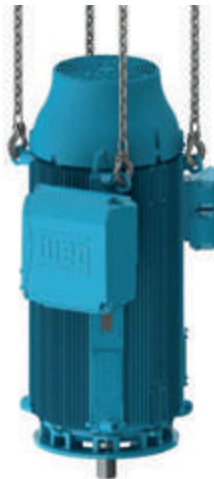
Figure 4.8 - Lifting of HGF and W50 motors.
