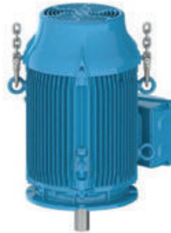
Figure 4.16 - Install the first pair of eyebolts
