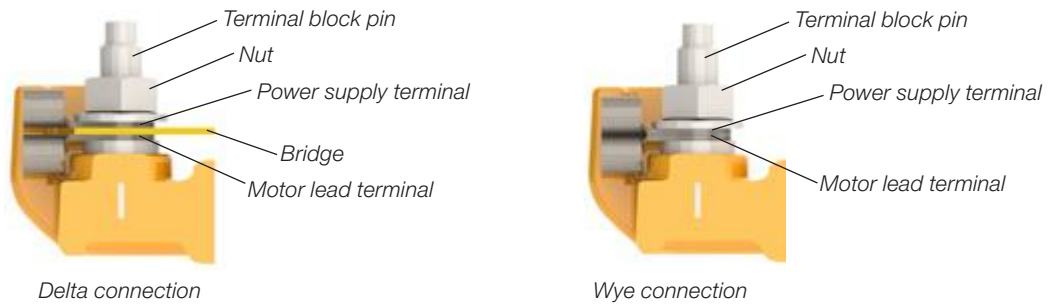
Figure 6.13 - Connection for W21 and W22 motors with terminal block
