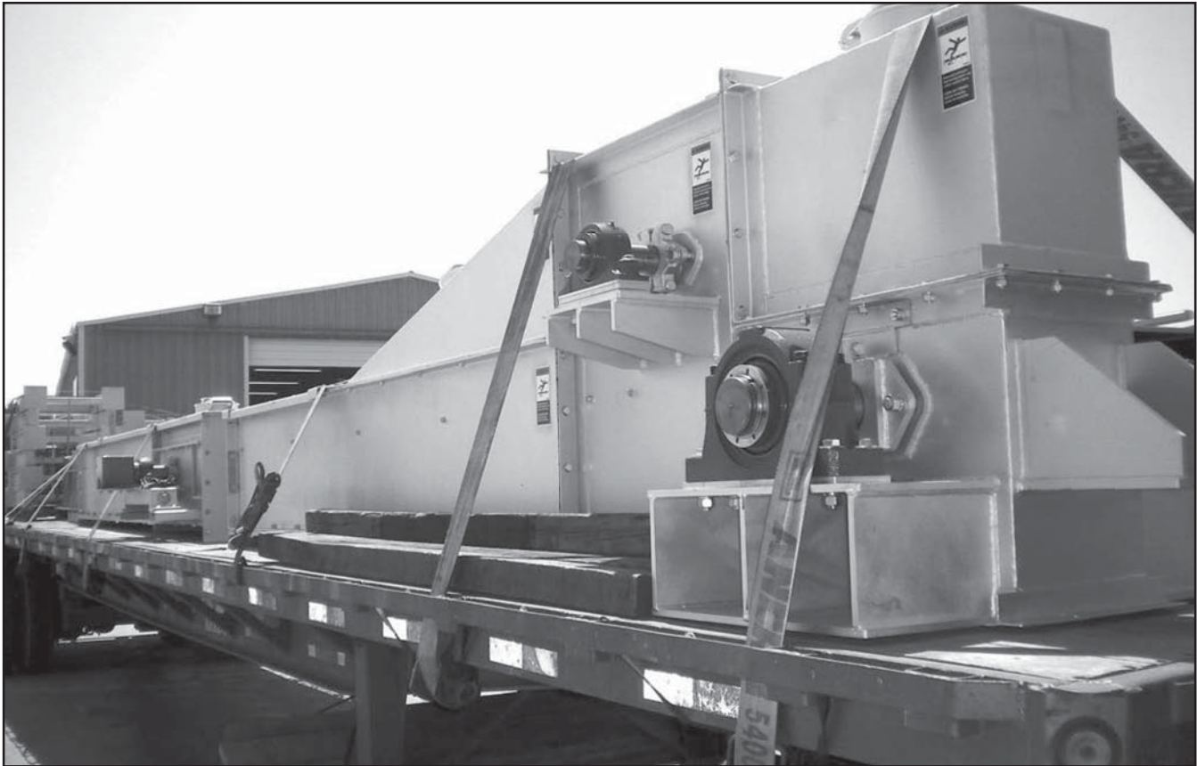
MSC Super Capacity Drag Head with Slack Side Tension Idler Sprocket
